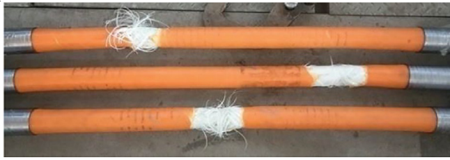
Fig. 10. Failure modes of the specimens.
