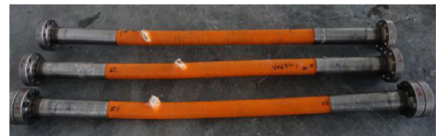
Fig. 14. Test specimens after burst.
