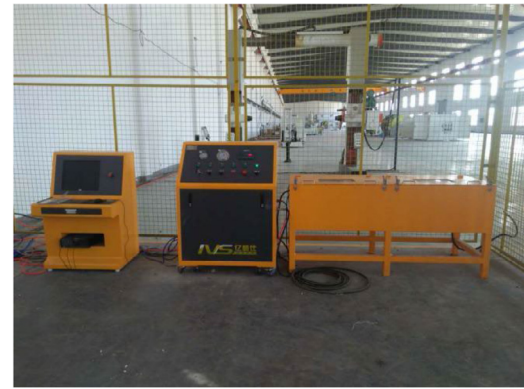
Fig. 12. Short-term burst pressure test system.
