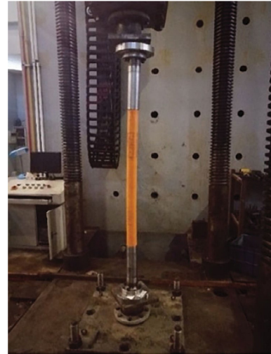
Fig. 8. Tensile test of a specimen.
