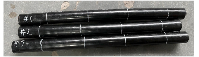
Fig. 16. Cable specimens for bending test.
